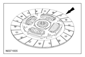
2. Check for a worn clutch disc lining. Measure the minimum allowable depth to the rivet heads with a slide caliper. Install a new clutch disc as necessary.
